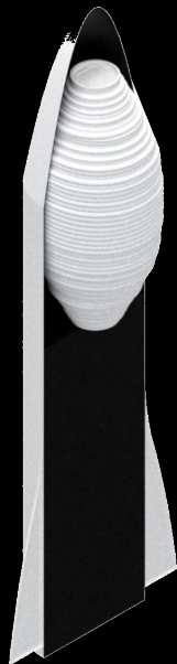
BFR Cargo Fairing Volume: 780 m 3 Weight: 70,000 kg
